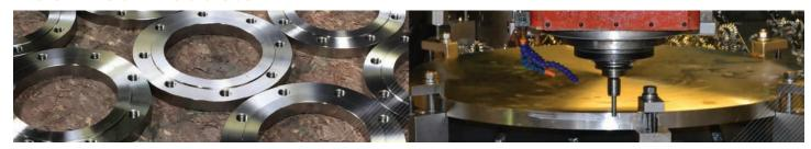
The quality of Stainless Processing, Inc.'s machined plate parts really separates us from the competition. Our ability to machine up to 120.00" OD covers virtually all of our customers' needs, and the possibilities are unlimited when it comes to machining circular items in our full-line machine shop, with standard tolerances of 1/32" or closer upon request.
